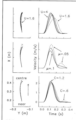
**FIGURE 12.** Effects of varying central control parameters on simulated kinematics. Sensitivity of predicted kinematic patterns to variation in central control signal parameters. Note, for the C command, paths are shown corresponding to C = 1.2 and C = .6 (dashed).
