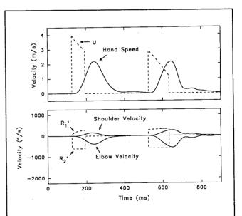
FIGURE 8. Effect of limiting the rate of joint equilibrium shift. Simulated near → center and center → far motions in which rate of EP shift was controlled at the joint level. The EV of the elbow was constant, and the shoulder EV was adjusted such that the hand EP shifted in a straight line toward the target.
