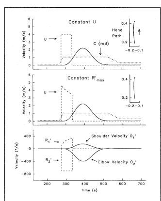
**FIGURE 5.** Simulated central commands and kinematics for near—center motions. In the simulation shown in the top panel, the hand EV (U) was constant at 4 m/s. In the simulation shown in the bottom two panels, the joint EVs (lower panel, dashed) were limited to  $\pm$  700°/s. In both simulations, the form of the hand speed profile (top two panels, solid) and hand path were similar to those observed empirically. The vertical axis also represents the amplitude of the C command in radians.
