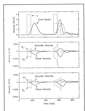
FIGURE 7. Simulated near→center and center→far motions. The top panel shows rates of hand EP shift (U) and predicted hand speed profiles. In one case, U was 4 m/s for both movements, and in the other, U was reduced to 2.2 m/s for the center→far motion. Joint EVs and predicted velocities corresponding to these two cases are shown in the middle and bottom panels.
