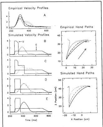
FIGURE 11. Effects of ISI on hand kinematics. Empirical and simulated hand speed profiles for single-step near—center (dashes) and near—right (solid) targets and double-step near—center—right targets with ISIs of 20 (dash-double-dot) and 60 (dotted) ms.
