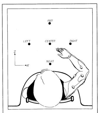
FIGURE 3. Top view of a subject sitting at the experimental table. The positions of the five target LEDs are shown. Five markers used to record the trajectories of the hand and arm can also be seen.
