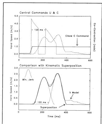
**FIGURE 9.** Simulated velocity profiles. Top: Central commands and predicted hand speed profile for a simulated motion to the near $\rightarrow$ center $\rightarrow$ far target. Bottom: Comparison of the  $\lambda$  model with superimposed minimum-jerk trajectories.
